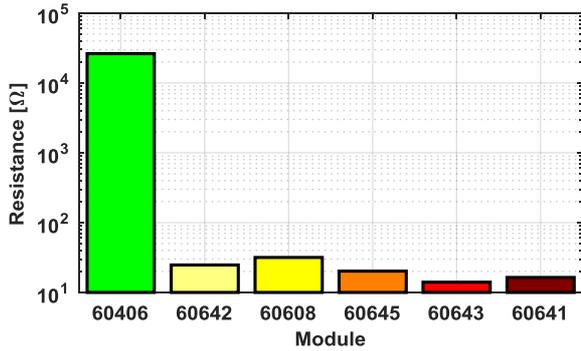
Fig. 9 Shunt resistance values determined from the IS measurements illustrate the same picture as the other characterizations. The PID modules have an  $R_p$  much lower than the typical value for c-Si PV panels, which is around few k $\Omega$ .
