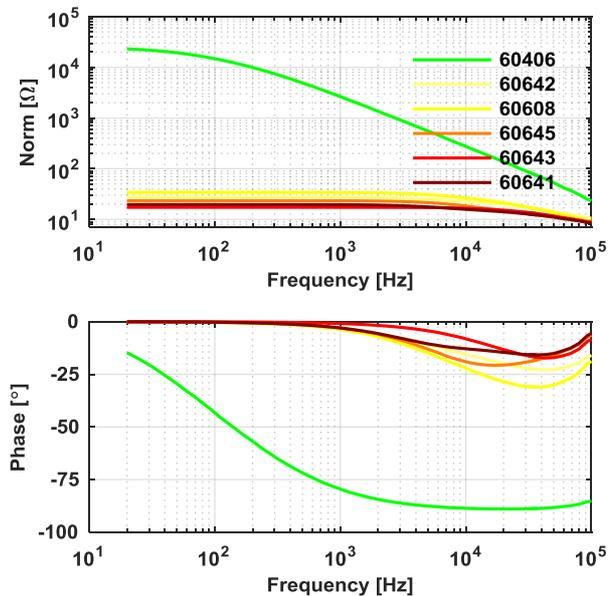
Fig. 8 Impedance spectra of the six PV modules, measured in dark condition in a frequency range from 20Hz to 100 kHz. The difference is evident between the best performing module (60406) and the others.
