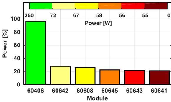
Fig. 4 Decrease of STC  $P_{max}$  of the modules relative to their datasheet value. It can be observed that the best performing module has an expected loss in power of around 1% per year from the rated value, while the other worst performing modules have an indisputable degradation problem.
