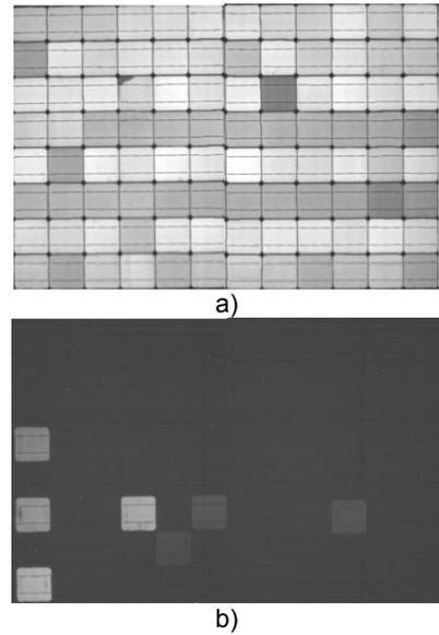
Fig. 7 EL image of a good panel, a) module 60406, versus a degraded panel, b) module 60608, taken in low current bias conditions.
